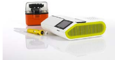
Figure 1 POCKIT™ Nucleic Acid Analyzer is a portable PCR amplification and detection system based on iiPCR technology.
