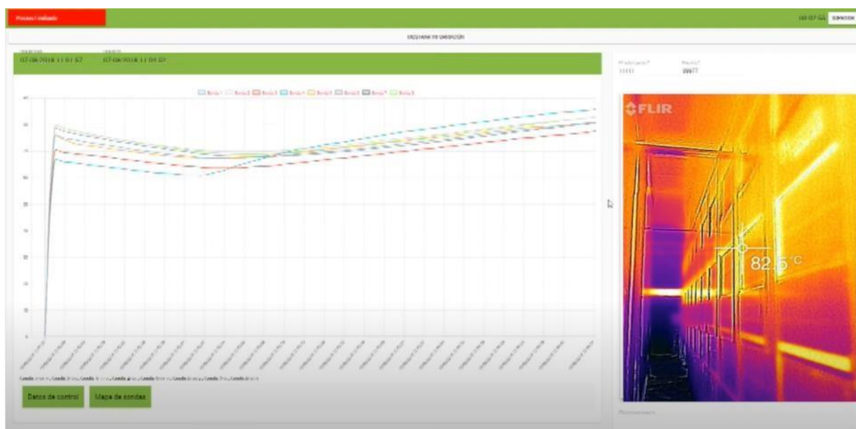
Figure 23. Thermal disinfection of a truck and data generated on the process
